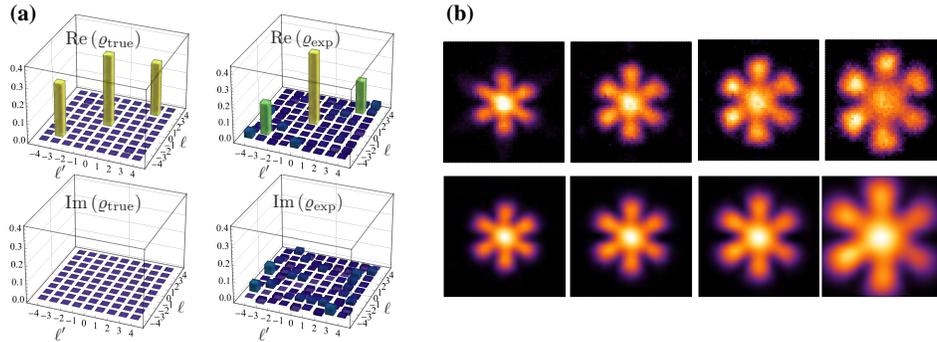
Fig. 3. Experimental reconstruction from compressed sensing. (a) Density matrix of the true state and (b) Reconstructed density matrix after two intensity scans with a signal space spanned by  $\ell \in \{-4, \dots, 4\}$ . The upper row shows four experimental ICCD scans at the planes  $z/z_R = 0, 1/3, 1/2$ , and 1, respectively. The lower row shows the predictions from the reconstructed state of the same ICCD scans.
